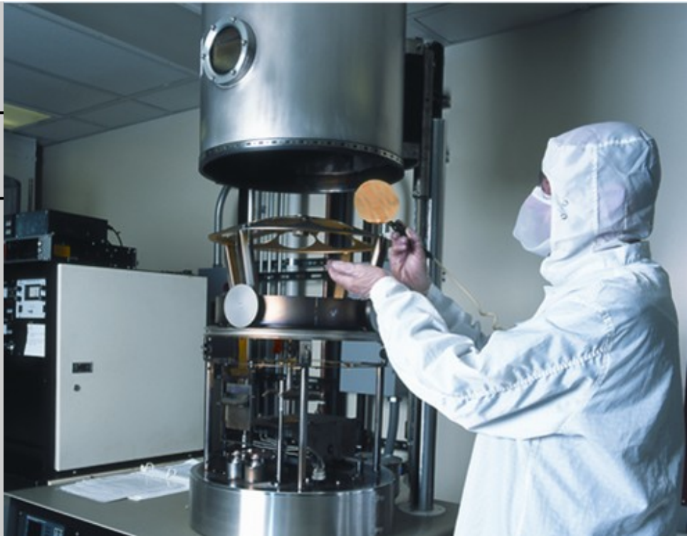
A thin film of gold is vacuum deposited on a 4-inch silicon wafer using a CHA electron-beam evaporator at the microfab lab. Photo courtesy Washington Technology Center
